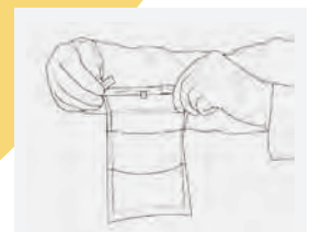
Bend wires in to seal.
