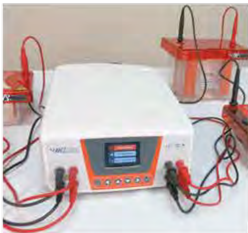
Four pairs of outlet terminals
