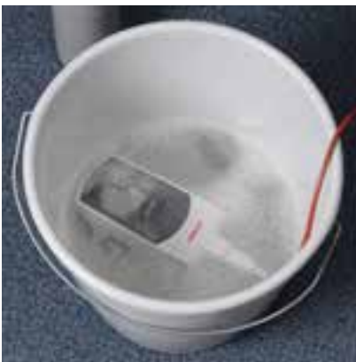
TF 410 - still working, thanks to IP67
