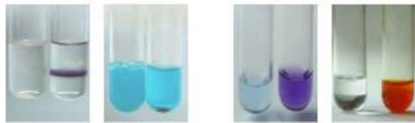
1. Benedict's test for reducing sugars 2. Benedict's test for reducing sugars 3. Biuret test for proteins 4. Biuret test for proteins
