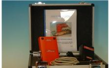
EXHAUSTIVE RESEARCH HAS CULMINATED IN THIS NON DESTRUCTIVE, AND NON INVASIVE INSTRUMENT, AS AN ACCURATE AND RAPID METHOD OF OVERCOMING THE PROBLEMS OF EVALUATING THE RELATIVE FRESHNESS OF WET FISH.
